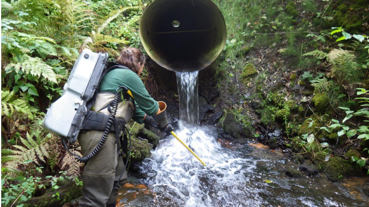
Figure 7.1 United States Fish and Wildlife Service (USFWS) scientist surveys for fish below the Atwater Rd culvert to interpret the impacts of culverts on the native fish population (Source: United States Fish and Wildlife Service).
